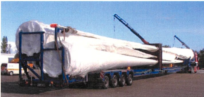
Figure 2: Example: The transportation of 3 x 45m wind turbine blades on extendable trailers
