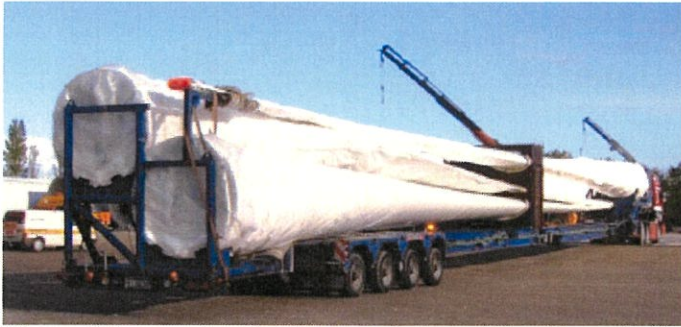
Figure 2: Example: The transportation of 3 x 45 m wind turbine blades on extendible trailers
